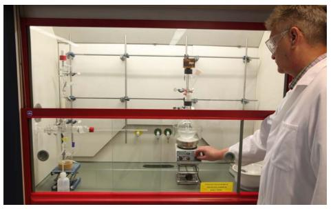
Fig. 3 Fume hood with work performed through the divided sash
