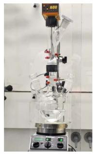
Fig. 9 Automatic powder dosing funnel on a three-necked flask for constant dosing over long periods of time
