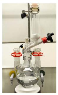
Fig. 8 Manual powder dosing funnel on a three-necked flask
