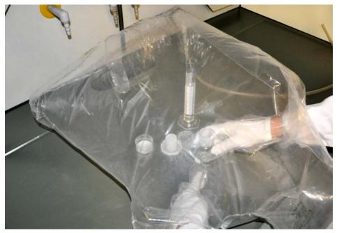
Fig. 14 Glove bag with closing clip for feed opening
