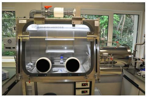
Fig. 13 Glove box with airlock
