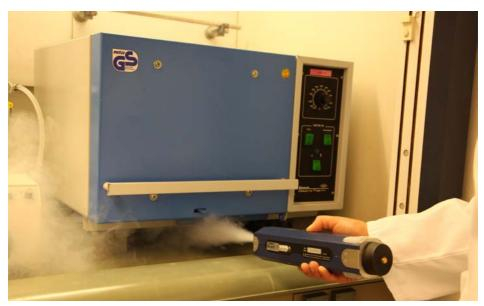
Fig. 4 Testing the fume hood with a smoke generator
